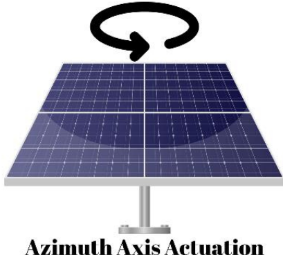
Fig: 10 Azimuth axis actuation of solar panel assembly
