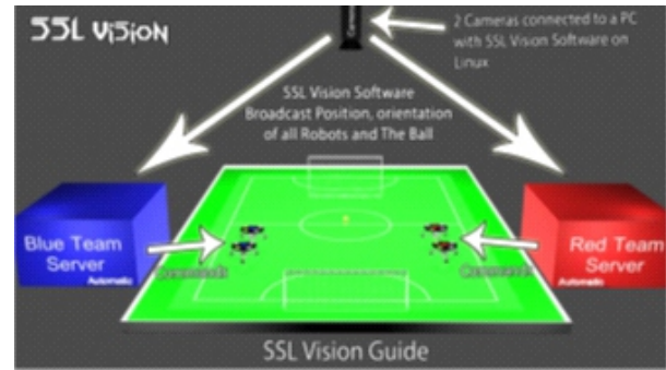
FIG. 2. OVERVIEW OF THE SHARED VISION SYSTEM USED BY THE ROBOCUP SMALL SIZE LEAGUE [15]
