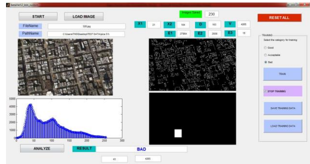
Figure 18: Software classifying Bad Landing Site successfully
