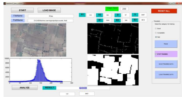
Figure 17: Software classifying Good Landing Site successfully
