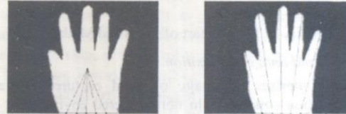
Fig. 6: (a) Hand Wrist Points Detection (b) Finger Tips Detection
