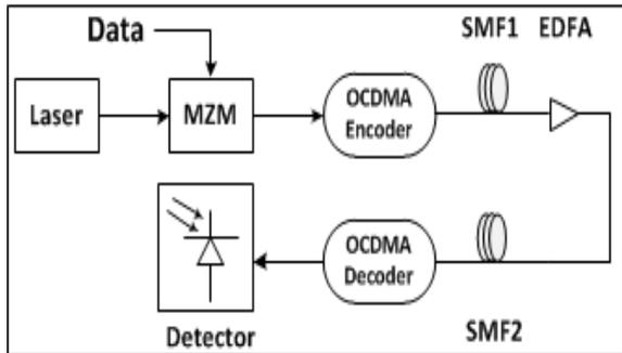
Fig. 3 Simulation setup for OCDMA LR-PON
