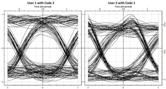
Fig. 6 Eye diagram of users with Codes reversed
