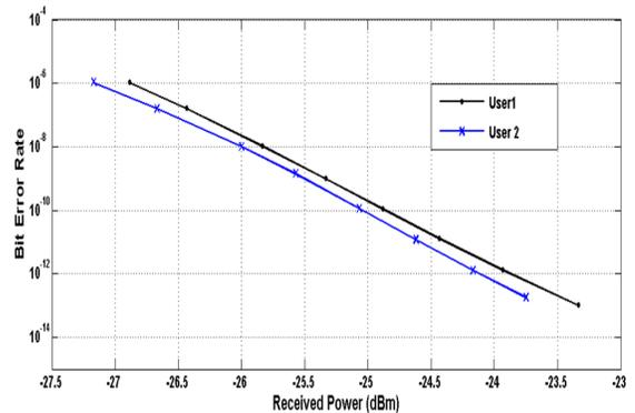
Fig. 4 BER diagram for two users
