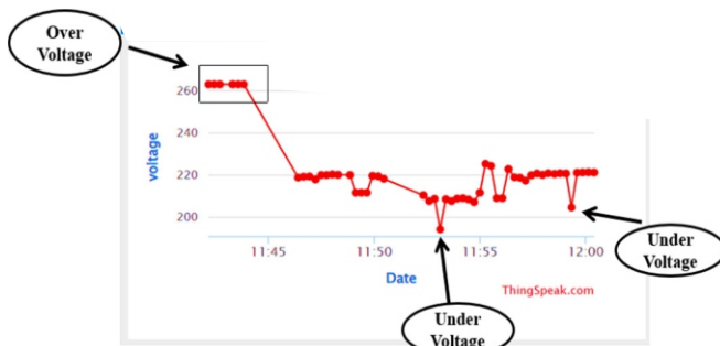
Fig. 11. ThingSpeak monitoring during over-voltage and under-voltage operating conditions.
