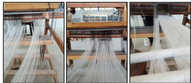
Fig. 3. Manufacturing of woven temperature sensors using a manual dobby handloom. pattern
