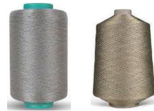
Fig. 2. Silver-coated polyamide conductive yarns used as sensing elements: (a) Shieldex® 235/36 (single-ply) and (b) Shieldex® 117/17 (single-ply)
